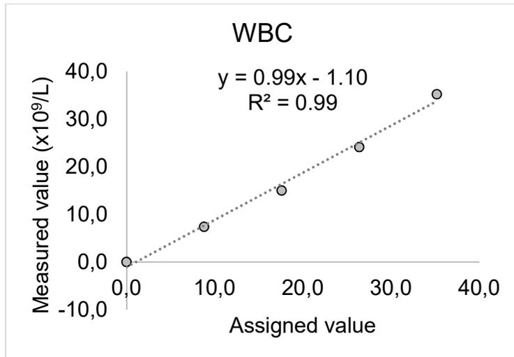
**Figure 1.** Assay linearity for Hb, Hct, RBC, WBC and Plt in Sysmex XN-1000. The linearity test was carried out with different dilutions made from samples with high concentration of each analyte, measured in triplicate. Hb – haemoglobin. Hct – haematocrit. RBC - red blood cell. Plt – platelets. WBC - white blood cell.
